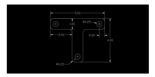
Reproduce the features described in the sample provided. First, create the lines, outlining the object. Fillet between these lines or use arcs to create the corners. Place the holes in their proper location. Dimension as shown. Place in title block.
